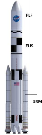
Figure 12. SLS Block 1B with EUS and 8.4 m PLF. (Image credit: The Boeing Company)
